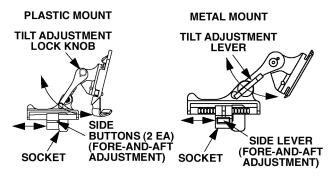
Figure 2-28. Tilt and Flip-up Mechanisms.
